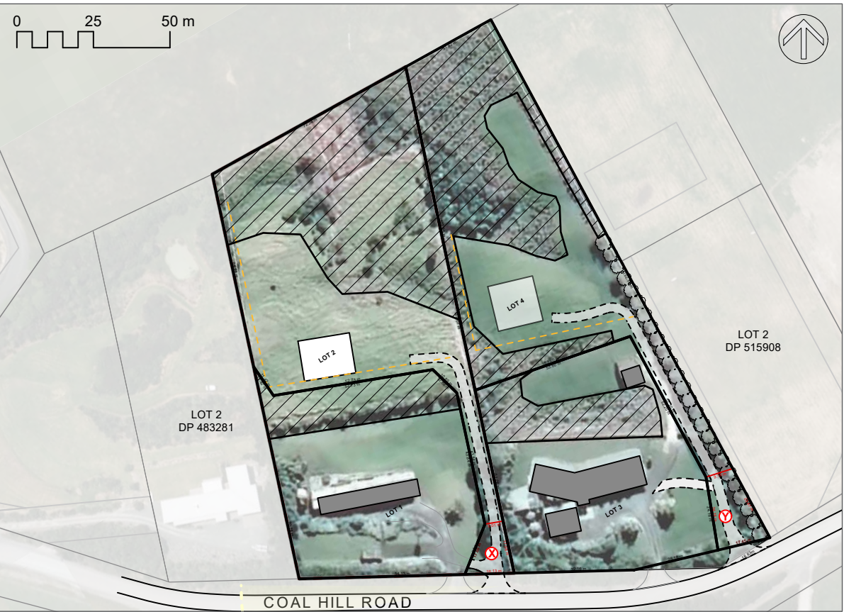
SITE PLAN OF TRAFFIC SIGHT LINES AT VEHICLE CROSSING - SCALE 1:800@A3
